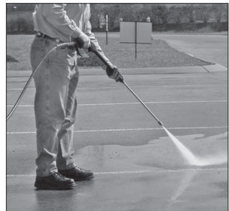
Figure 14 - Optimum angle to cleaning surface
