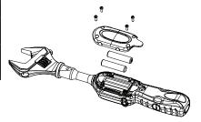
**ATTENTION:** When opening the battery cover of your wrench, you can see a viewing window for the **water contact indicator**. Through this viewing window, you can check if this wrench is damaged by water penetration where the water contact indicator turns red.
