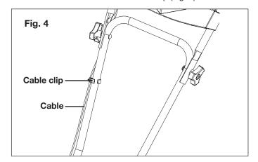
**WARNING!** Make sure all handle knobs are properly tightened before using the electric tiller + cultivator.
