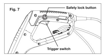
2. To switch OFF, release the trigger switch (Fig. 7).
