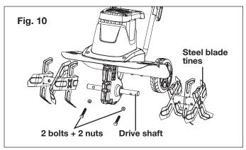
**IMPORTANT:** The tines must be set in the correct turning direction. Note the way the old tines came off and replace the new ones exactly the same way.
