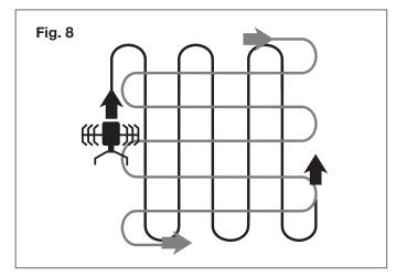
Pay special attention when changing direction. Apply light pressure to the handle in order to lift the tines and facilitate the turn. Turn the product around using the wheels as a guide. Gradually release pressure on the handle and move the tines back to the ground.
