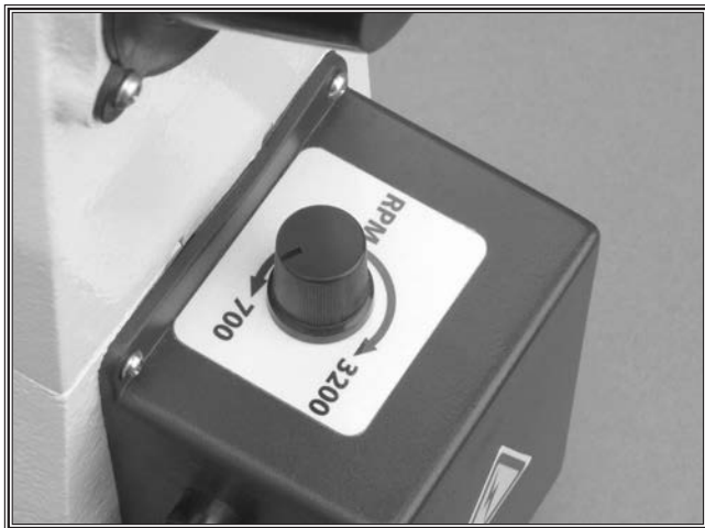
Figure 16. Speed dial turned all the way down to the lowest speed.
