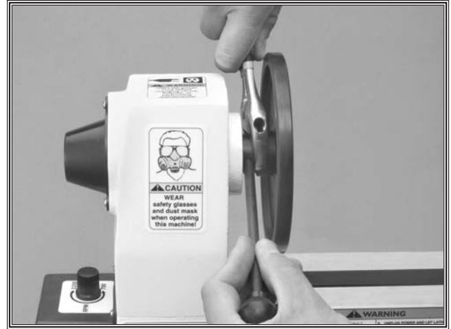
Figure 11. Tightening face plate to headstock spindle.
