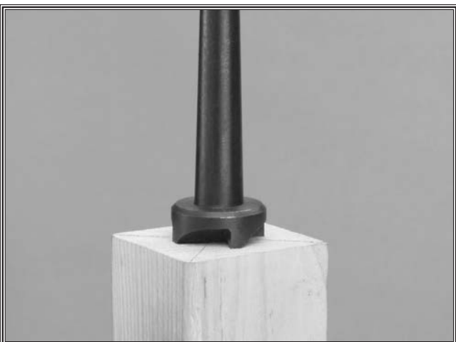
Figure 25. Spur center properly embedded into workpiece.
