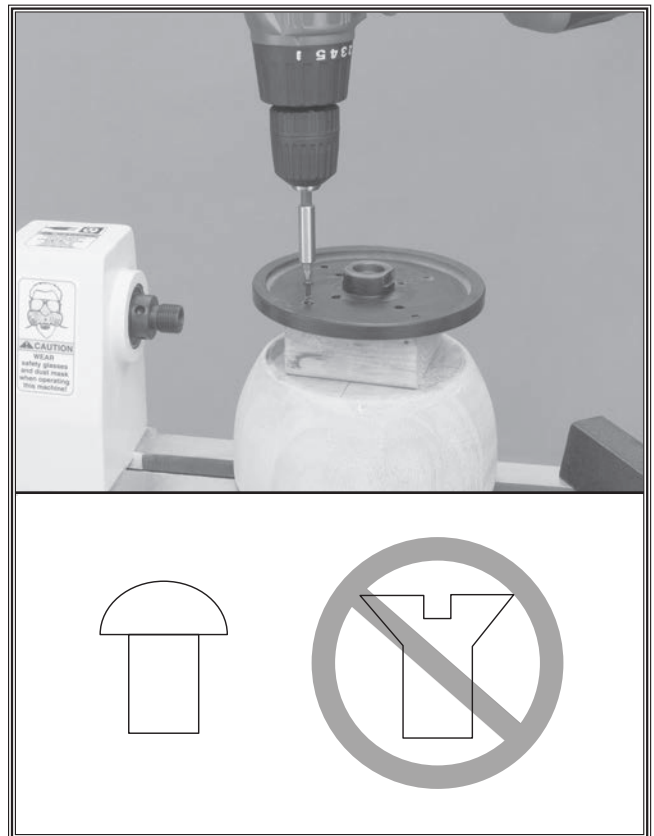
Figure 27. Mounting face plate to a backing block, which is glued to the workpiece.
