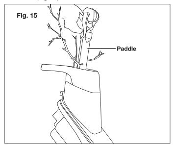
⚠WARNING! Never put your hands into the hopper while the wood chipper + shredder is running. Always use the paddle supplied with your shredder to push items into the hopper.
