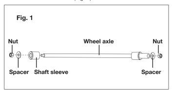
2. Insert the wheel axle into the shredder stand assembly, and re-assemble the shaft sleeve and the support cover (Fig. 2).
