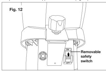
3. To power the wood chipper + shredder off, push the removable safety switch to the OFF position. To disable the machine, remove the safety switch completely (Fig. 13).
